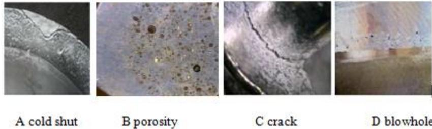
Figure 1 Defects in aluminum alloy castings [9]
